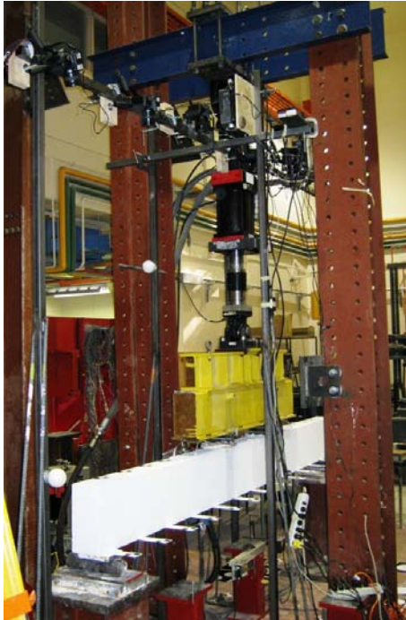
Figure 1. Example of the camera system positioned on a metal frame above a concrete beam
