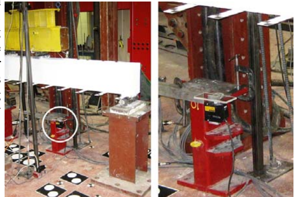
Figure 3. Example of a 1D laser transducer positioned under a beam being tested
